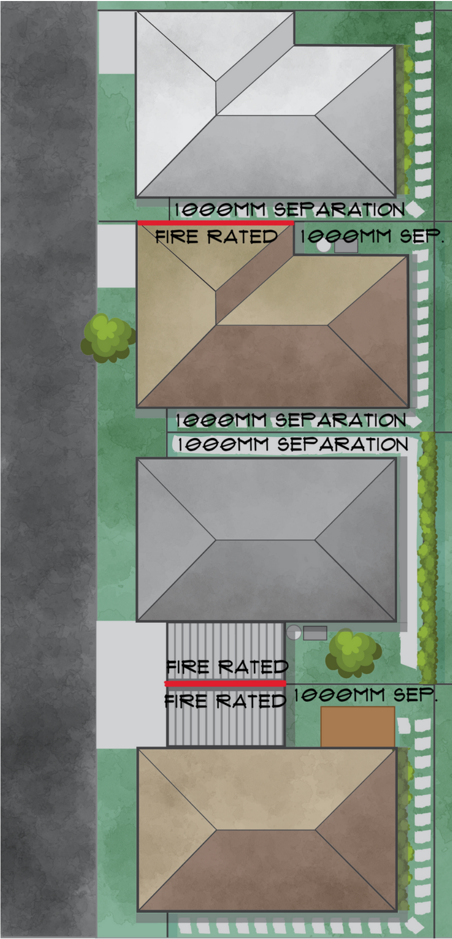
Figure 15: Fire separation between structures.
