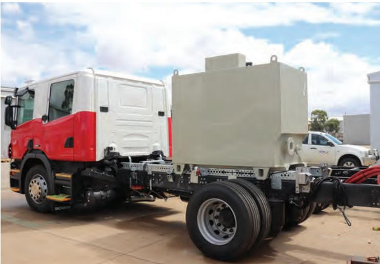
When phase one of the build is complete, a crane lifts the lockers onto the pumper, where they are bolted into place and extra compartments affixed.
