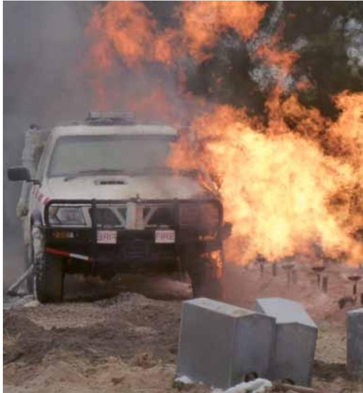
**Left:** Flame immersion of ultra-light tanker test vehicle on bushfire flame front simulator
