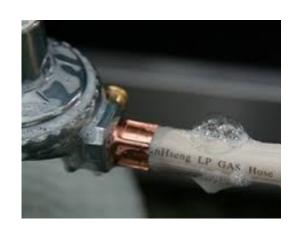
The gas bottle hose is being soaked in soapy water, to see if there are any leaks. If there is a leak, the hose should be replaced.
