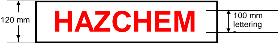
Figure 11: Form and dimensions of an Outer Warning Placard
