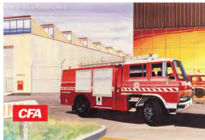
Right: The 3000-litre Hino 3.4D tanker was designed in 1986 on a GT175 4X4 chassis and included five-speed manual gearbox and power-assisted hydraulic brakes. The 3.4D had a built-in roll over protection structure on the rear deck.
