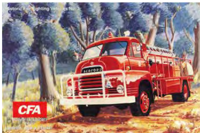
Right: The RLHC series Bedford Type 4.4 tanker was popular in the 1960s. It carried 3,600 litres of water and included a deck-mounted monitor and a VW Godiva pump at the rear.
