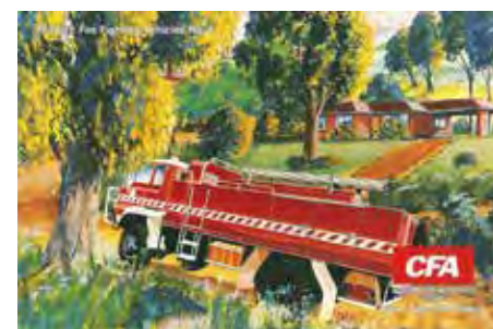
Right: The 3000-litre Hino 3.4D tanker was designed in 1986 on a GT175 4X4 chassis and included five-speed manual gearbox and power-assisted hydraulic brakes. The 3.4D had a built-in roll over protection structure on the rear deck.
