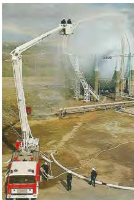
Left: The hydraulic platform was designed and built in Australia on an International truck chassis. It had an articulated steel boom mounted on a rotating turntable. The boom could reach heights of 22 metres and could deliver 3,600 litres of water per minute.
