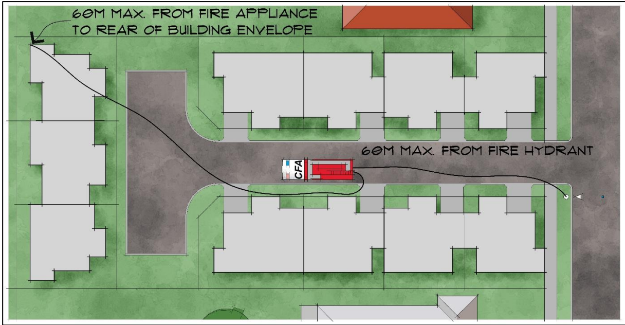
Figure 9: If building envelopes (or buildings) are provided.
