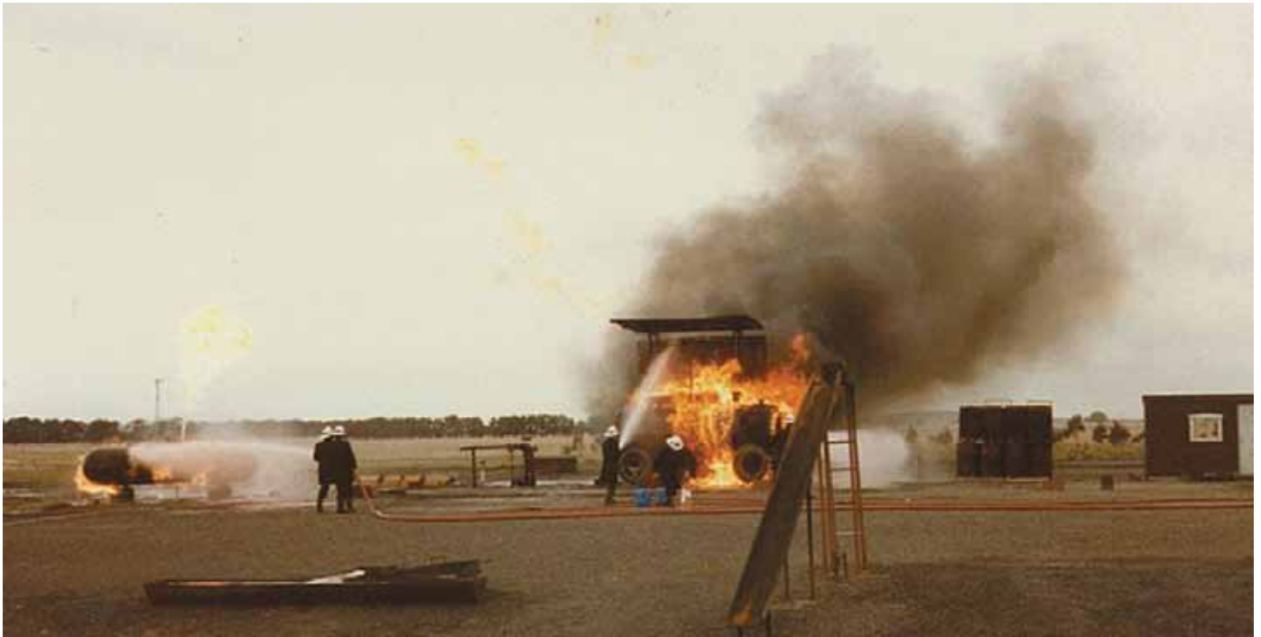
Figure 5.4 Comparative photograph of drills on the flammable liquid PAD. The bullet prop on the left uses LPG; rail car prop in the centre burning flammable liquid, 1984. Photo courtesy of Peter Baker.
