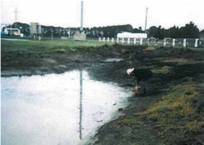
PAD operator pouring approximately 5 litres of petrol on to the surface of the dam to 'prime' it.
