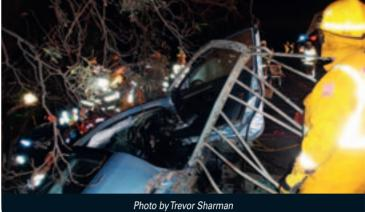
The vehicle was very unstable and there was a risk it would slide into the creek, so multiple security points were fixed to the car using chains and winch lines.
