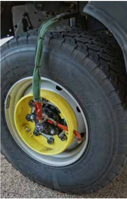
Left: Wheel with inflation/deflation device fitted
